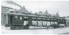
To fight germs, sleeping-car bedding was given "sun baths," as demonstrated in this August 1906 photo of a wooden 12-section/11-drawing-room car at the Pullman plant in Chicago.
