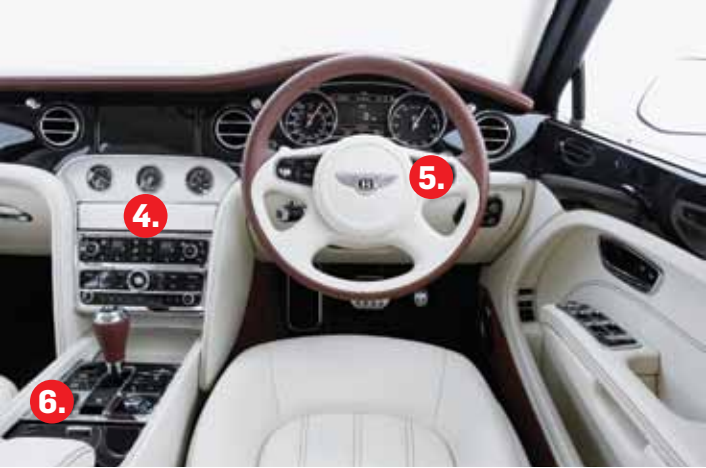
4. This retractable, jack-equipped drawer cradles a custom iPod (whose screen displays the Bentley wings when it's not being used). 5. Clutch-impaired speed demons can use the paddle shifter —and fool their chums into thinking they can drive a standard. 6. This chrome dial adjusts the car's suspension, so you can either “float” along the road or feel like you’re taking the Dunlop Curve at Le Mans. 7. The Mulsanne’s front-end styling pays homage to the enormous headlamps and commanding vertical grille of Bentley’s 1930 8-Litre —just the sort of fun fact a young tech billionaire would love to drop.
